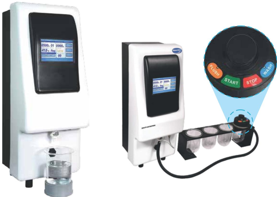
The PreCiFill is Compact, Transportable and offers quick and easy preparation of up to 10 litres dissolution media in less than 15 minutes. In a single pass the media for dissolution tests can be precisely heated, degassed and filled gravimetrically into vessels. Foaming media like SDS (Sodium Dodecyl Sulphate) can also be used.
