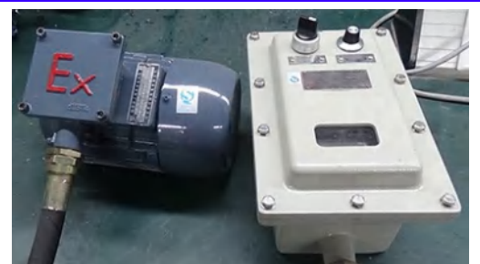
Ex control box
